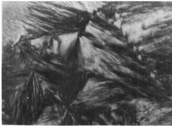
Figure 7. The initial domains in C_2 , at 65^\circ C , with d = 20 \mu m , \nu^2 = 0.9 \times 10^3 \text{ Hz}^2 , (E_{th}^{in})^2 = 121 \times 10^8 \text{ V}^2/\text{cm}^2 .
